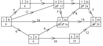
The arcs on the shortest route are those for which the difference in labelling at each end is equal to the length of the arc This gives the shortest route as ABCEFH, of length 29
